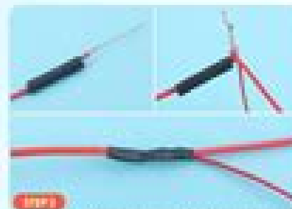
STEP 3 Referring to the circuit diagram of STEP2, first place the heat shrink tubing on the red wire, then connect the wire cores together, and then completely cover the wire cores with the heat shrink tubing. Bake the heat shrink tubing with a lighter to make it shrink.
